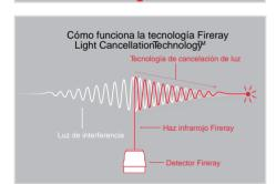
Light Cancellation Technology  $^{\mathbb{M}}$ . Fireray's patented technology actively blocks ambient sunlight or artificial sources and allows beam detectors to be installed in skylights and glass atriums without triggering unwanted alarms.
